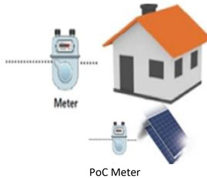
Figure 5: Representative Illustration of a Multi-Metered DER Configuration
