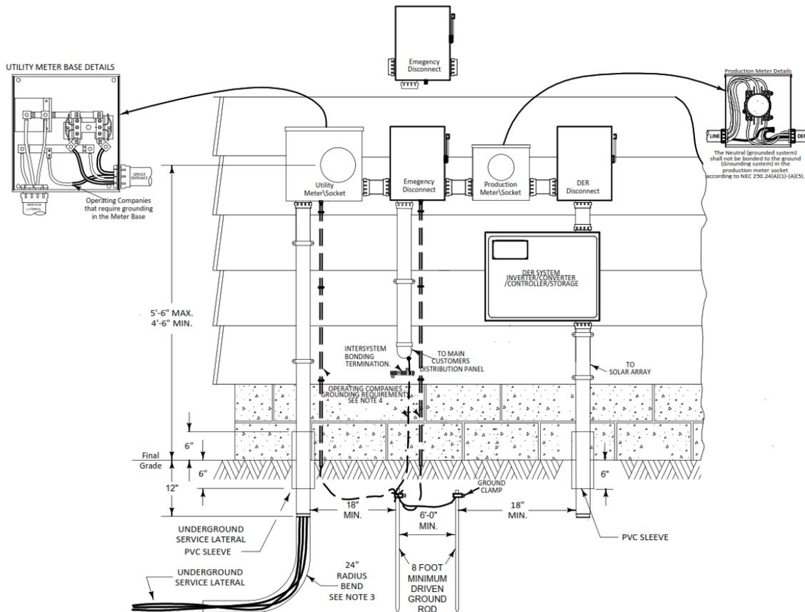
**Figure 6: DER Metering Installation Diagram for a Residential Multi-Metered DER**
