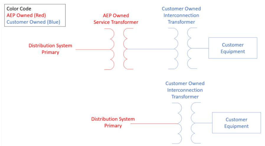
Figure 2: Service Transformer and Interconnection Transformer Examples
