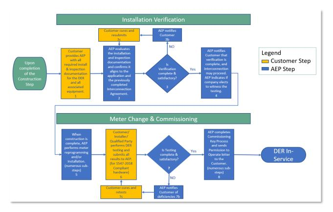
Figure 7: Process Flow for Commissioning-related steps of the DER Interconnection Process
