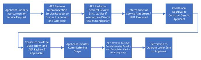
**Figure 1: Interconnection Application Process Flow**
