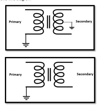
**Figure 3: Acceptable Single-Phase Transformer Connections**
